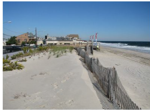
Figure 181 above shows the changes to the beach at 8 th Street in Ortley Beach since its initial survey in 1986. The dune has grown vertically, however losses to the dune toe and beach face resulted in a shoreline retreat of 16 feet and a net loss of 7.402 cu.yd/ft. of sand. Photo on the left was taken in February of 1989 and shows the view looking northeast from the boardwalk. Photo on the right was taken in October of 2011 and shows the view north from the crest of the dune.
